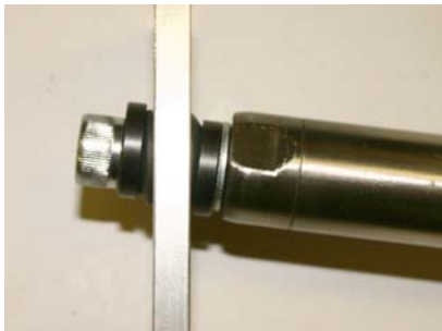
Function: Ball and socket washers adjust for angular offset between linear motor slider and Payload. (A spring washer should be used as well.)
